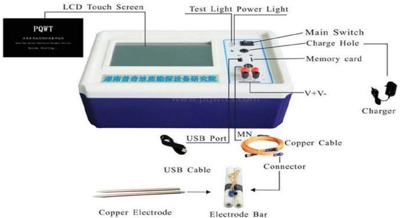
Fig. 3.1: Different parts of PQWT-W200
